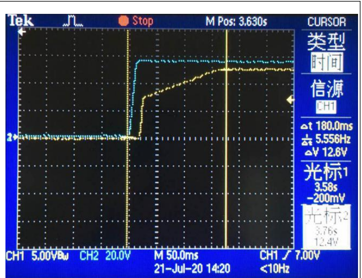
Output response & load (12V / 0.02A)
